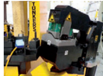
Power press unit for cutting of the component
