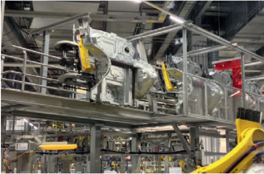
AFS Conveyor as infeed conveyor in a production cell with protective housing
