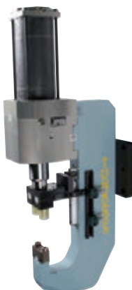
C-frame system as dual punch with multi-force cylinder
