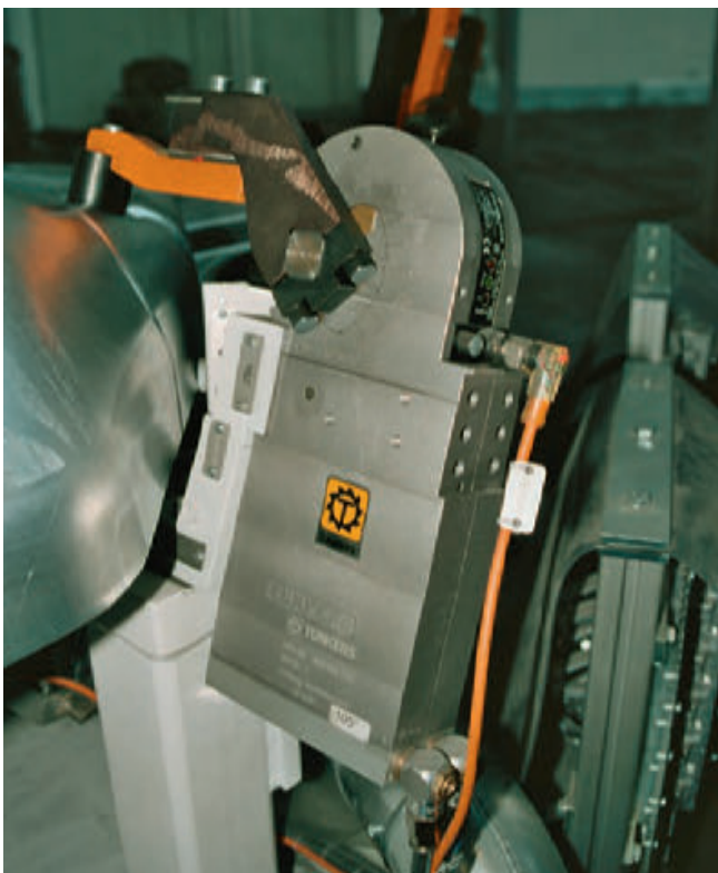
Detail: Alpha Gripper with contour pressure block
