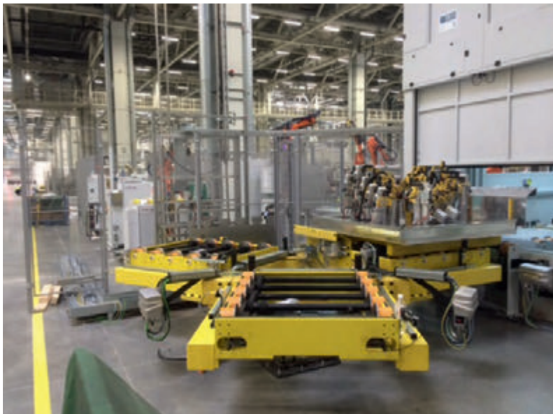
Tool storage zone on rotary table
