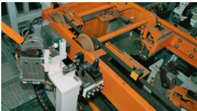
Underbody clamp for mounting the floor after the roller conveyor has been lowered
