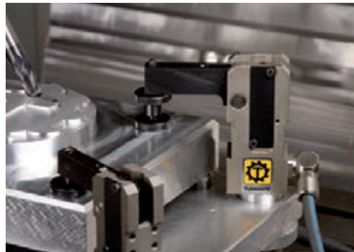
PKSG 20 in threaded form for clamping an aluminum component during the chip removal process
