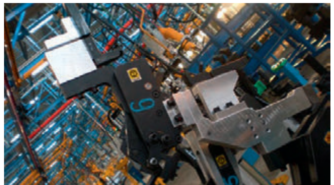
HKC 40 Manual Clamp in clamping fixture
