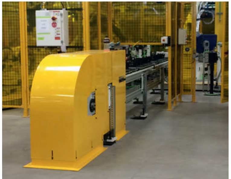
AFS 90° Conveyor as manual loading station for longitudinal parts
