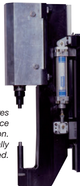
The installation of an additional external guide and anti-rotating device is recommended with extreme stroke lengths and the use of multiple tools. This can be realised in the form of a linear guide on the inside of the C-frame, or an external column guide.
