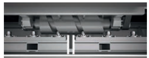
Floor mounted cam followers engaged in the drive cam
