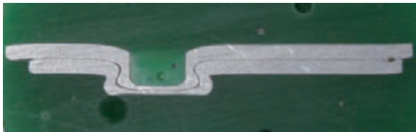
Cross-section of a clinched joint material: Aluminum 1.5 mm thick
