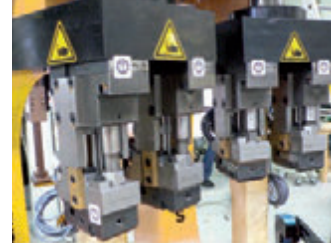
4 die heads for punch bolts
