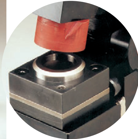
Pneumatic toggle-lever clamp for punching holes for 35 mm dia. pipe unions in sheet steel
