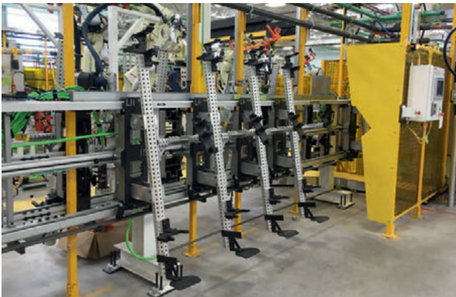
AFS 90° Conveyor as manual loading station for longitudinal parts
