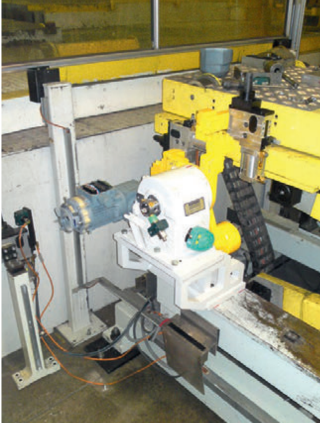
EXPERT 'Windmill' globoidal index drive with precision locking for floor clamping technology on transport tasks
