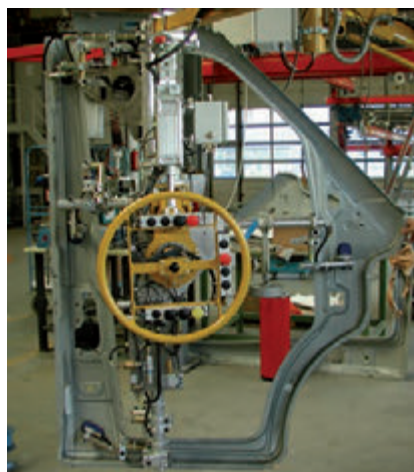
Manipulator gripper made from the Round Tube System (TRR)
