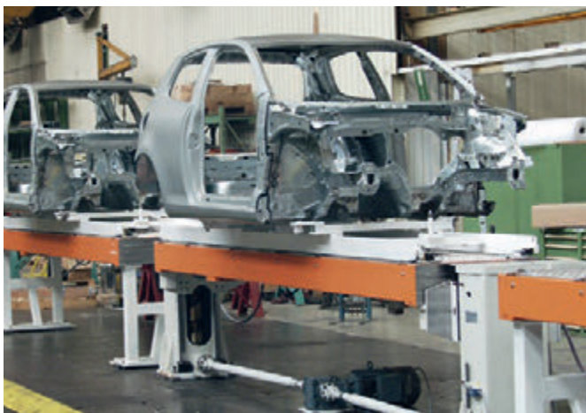
Lift powered rollerbed in upperbody line
