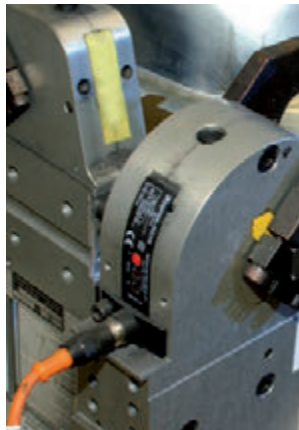
Position sensing cassette fitted to a knee-lever clamp
