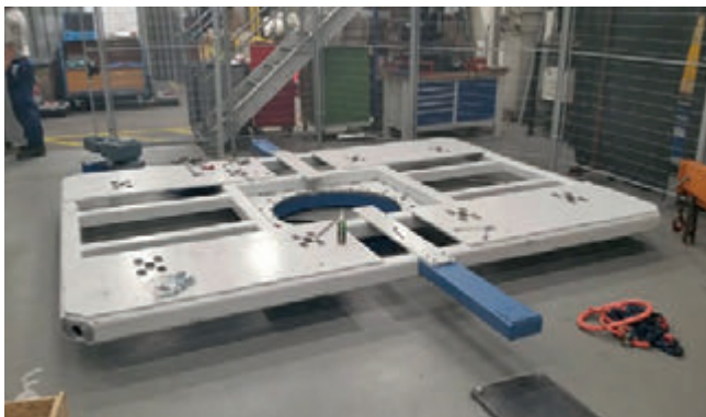
SOPAP Low-profile bin changeover system based on the TXR 1100, shown here for 2 bins
