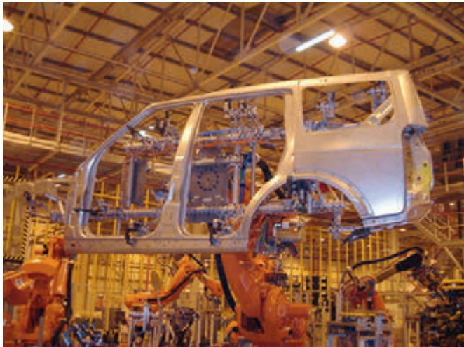
Gripper system for handling a body side
