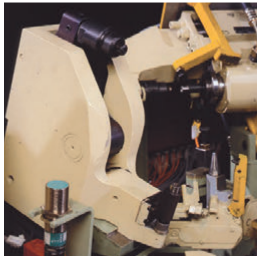
Power press unit with pneumatic drive
