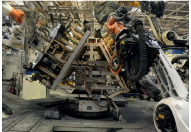
EXPERT Rotary Table, 2-stop positioning
