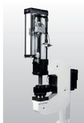
C-frame system with HydroAir cylinder
