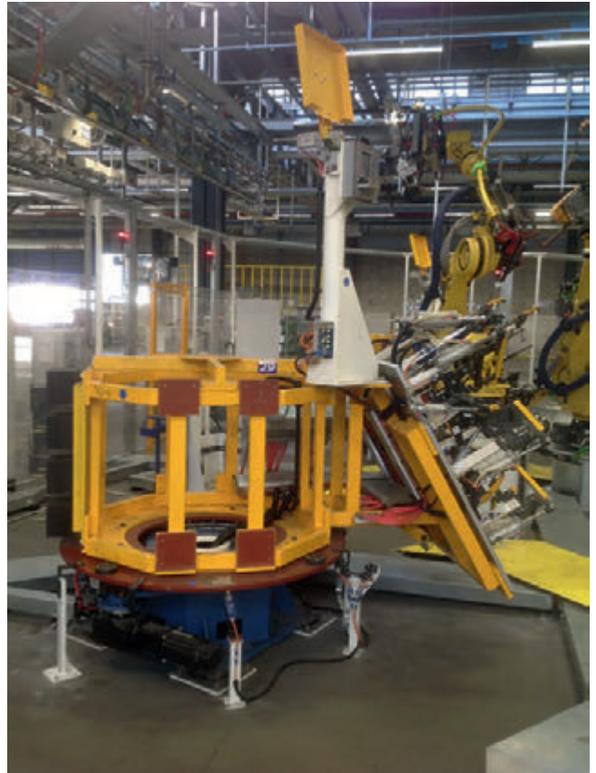
SOPAP TXE 1100 Tool unit in car body construction, flexible rotating fixture for tools
