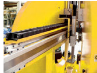
Linear unit for positioning of parts in the fixture
