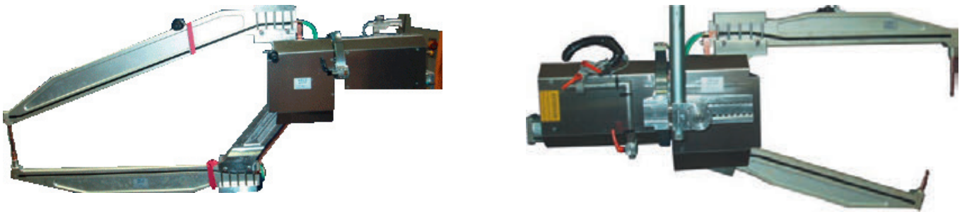
HD transformer weld guns
